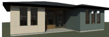
HIP ROOF - BACK VIEW
