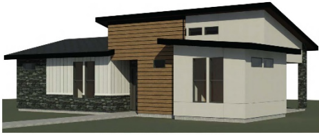
SINGLE SLOPE ROOF - FRONT VIEW
