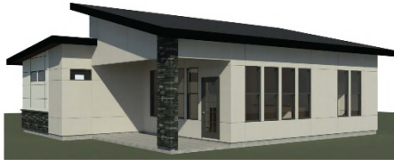
SINGLE SLOPE ROOF - BACK VIEW
