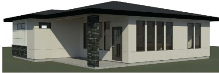
HIP ROOF - BACK VIEW
